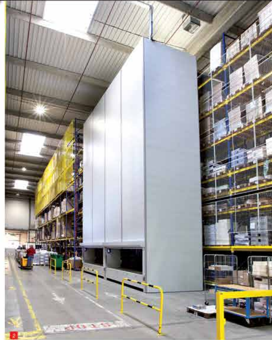
2. Two Storage Tower TOWER 500 FLAMMARION WAREHOUSE (Height : 11 meters) 3. et 5. Metallic dividers 4. Divisible Plastic Box 6. TOWER 300 Tray at the Pitié Salpêtrière HOSPITAL CENTER 7. TOWER with double access at the BONBONWEB WAREHOUSE
